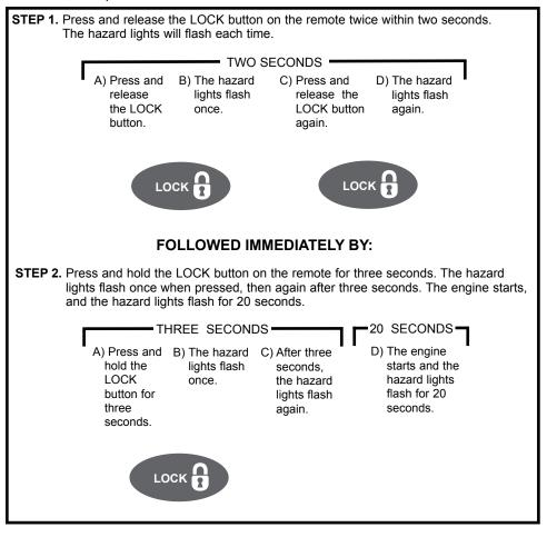
**NOTE:** Any vehicle started with the Remote Engine Starter can idle for a total of 20 minutes. Automatic engine shutdown occurs after 10 minutes, but the vehicle may be remotely started as many times as the user wishes and run for an additional 10 minutes. After 20 minutes of total operation, however, the vehicle must be started manually to reset the Remote Engine Starter.
